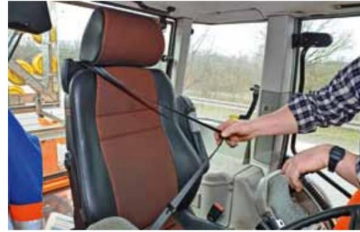
The three-point safety belt and the head rests provide more safety in road traffic.
