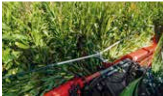
The infinitely adjustable header speed ensures a uniform crop flow, adapted to the forward speed of the forage harvester.
