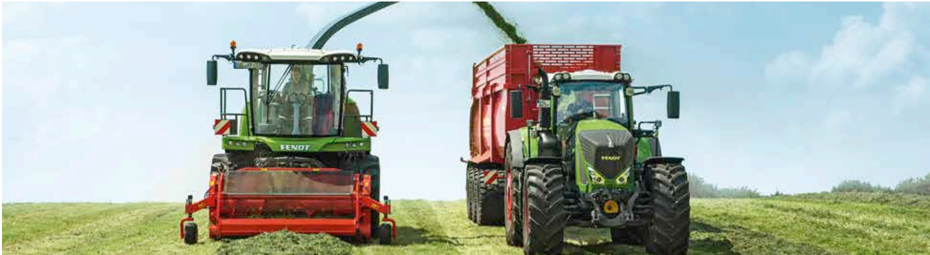
Crop feed over six feed rollers guarantees optimal pre-compression of the chopped material. The cutting length is infinitely adjustable from inside the cab.
