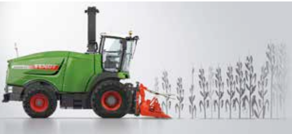
The maximum output control automatically adjusts ground speed to match the harvesting and crop conditions. It utilises the engine power optimally.
