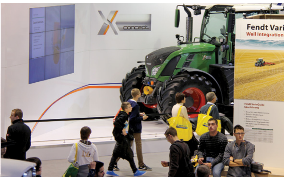
Bottom left: The Fendt exhibit featured the X Concept tractor – the result of Fendt design and engineering to develop a tractor with an integrated electric generator that could be used to power implements and attachments. In the future, tractors and implements could be more efficient and more flexible to configure than is possible today with the mechanical PTO and hydraulic systems that provide power from the tractor to implements and attachments.
