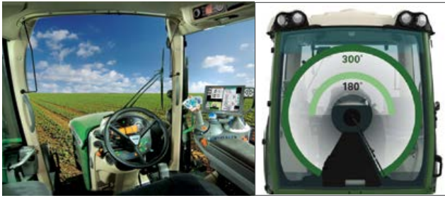
New Fendt 700 Models feature optional segmented windshield wiper with 180° and 300° wiping (standard on 800 and 900 Series).
