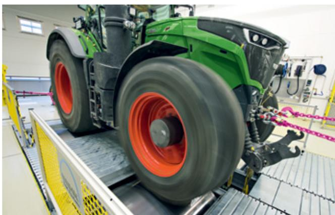
Top photo: The standardized pink chains can withstand forces of up to 22 tons. Above: The distance between the axles can be flexibly adjusted from 6½– 19½ ft, which ensures that all tractors can be tested – from the 200 Series to the 1000 Series.
