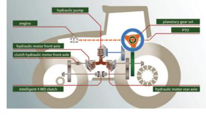
"With the 1000, Fendt also developed a completely new drive train integrated with a new CVT," Keeney explains. "The concept is called VarioDrive. Up to now, the rear and front axle, when engaged, were supplied with torque in a fixed ratio. However, on the 1000 Series, the front axle is now driven by a second, separate transmission output independent of the rear axle.
