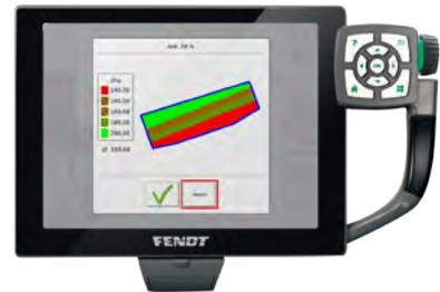
An application card can be transmitted to the Fendt machine from a field database or farm management information system (FMIS) via the ISO-XML data format using VarioDoc Pro (via USB, Bluetooth or GSM). However, the implement must have ISOBUS and the software activation to communicate with the tractor.
