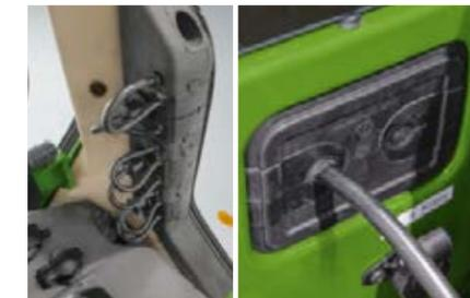
Fendt offers a clever solution for cables that run from the rear or front of the tractor into the cab. Cables of any size can be guided through the special lead-throughs. The rear window can keep closed, so dust, dirt, water and noise stay outside.
