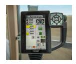
All the general functions including the LoadLogic weight management system, tyre inflation system, fan control, machine folding/unfolding system and the toolbar lift/lower mechanism - are operated via ISOBUS. You can monitor the level of the seed and fertiliser tank on the ISOBUS screen.
