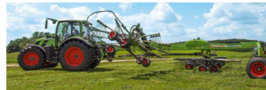
The sequence control always lifts the Fendt Former hay rake rotor on the headland in just the right sequence.
