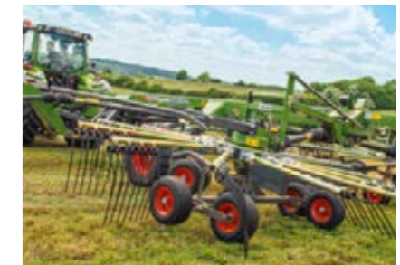
When lowering on headlands, the back wheels touch the ground first, followed by the front wheels. When lifting, the rotors are raised first at the front. This Jet-Effect protects the sward.
