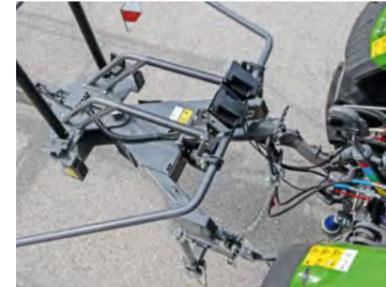
Rear-shifted pivot point and shorter frame length for outstanding manoeuvrability – despite the larger working width.
