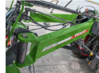
For transport, the rotors are hydraulically folded and mechanically secured.
