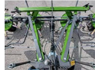
The three-point tower with three-material bearing bushings in the folding hinges is both durable and particularly maintenance-friendly.
