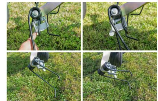
A simple adjustment of the tines on the outer rotor activates the edge-processing mechanism. This puts the tines in the innermost position for a neat field edge and to perfectly distribute the mowed crop.
