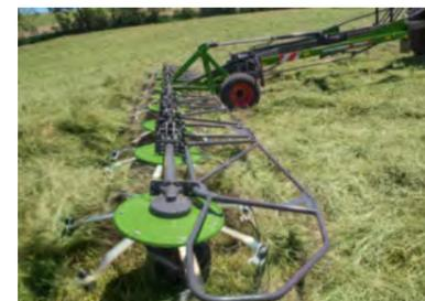
The large, forward-running transport wheels make sure it runs very quietly with a consistent working depth.
