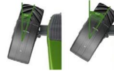
At the headland or during front loading work, you benefit from VarioActive steering, reaching a full wheel turn with just one steering wheel rotation. Up to 8 km/h the superimposed steering system is unrestricted, from 8 to 18km/h the superimposition effect is linear.
