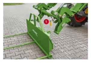
The implement is conveniently unlocked using a lever (1) on the quick-attach frame; it just takes a flick of the hand. When mounting an attachment, lock it automatically by tipping it back completely.
