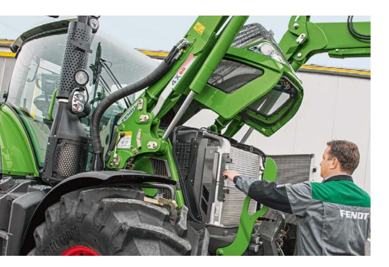
Maintenance even when the front loader is hitched Since the designs of the front loader and the tractor have been specially adapted to each other from the very beginning, all maintenance work can be performed while the front loader is mounted. This gives you easy access to the oil dipstick to check the oil for example. The front loader was designed to guarantee a very long service life through simple maintenance and the use of the best materials.
