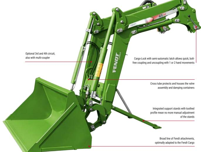
Life-time design for a long service life High-grade materials ensure durability for a long service life. High-strength fine-grain steel is the key factor behind the lifetime design of the new Fendt Cargo. In addition to high stability, it also guarantees a low weight. The Fendt profile, which is welded in one continuous seam, ensures high stability and therefore a long service life. The generously sized bronze bearing points with lubrication also guarantee a long service life and minimum wear.
