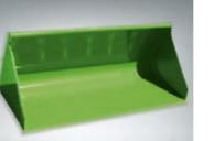
The light material bucket is available in widths of 2100 mm (1.27 m<sup>3</sup> flush volume) and 2400 mm (1.45 m<sup>3</sup> flush volume). The bucket is powder-coated instead of lacquered and the blade is made from durable, low-wear Hardox 500.
