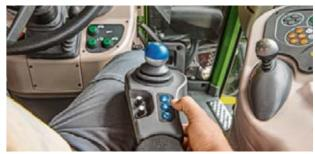
200 Vario: The electric crossgate lever (optional) controls the front loader with extreme precision. The 3rd and 4th control circuit can be operated without changing hands by using the push buttons on the crossgate lever. THE CARGO SWING ARM
