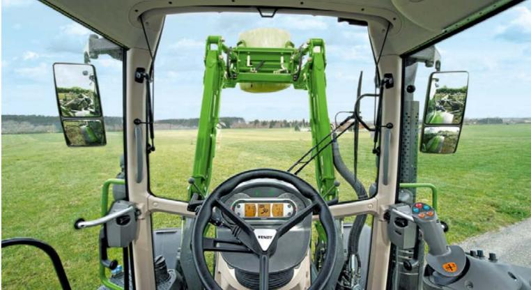
The tractor's uniquely curved windscreen always gives you a perfect view of fully extended implements. At the same time, its curvature prevents material from building up on the windscreen and keeps the view completely clear.
