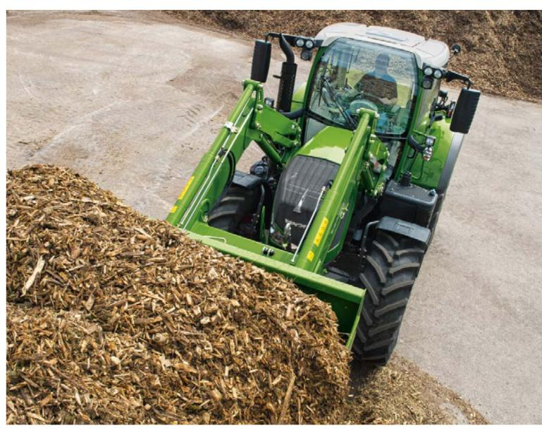
The front window opens out all the way, even with the front loader swing arm fully extended. Choose the right cab variant in the series.
