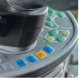
With the orange reverser lever, you can easily change directions with your left hand. Hold the lever down and the Vario stops. Release the lever and the tractor automatically drives in the preset direction.
