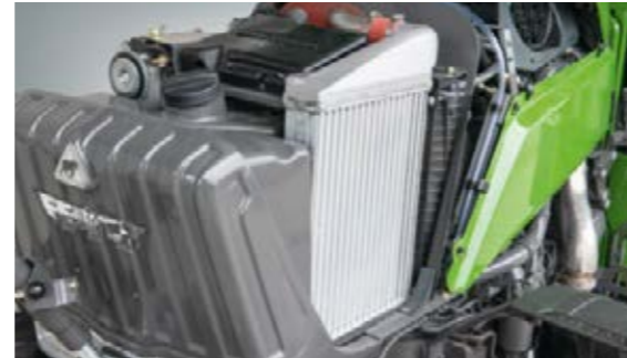
The cooling system has large intake areas with optimum air supply. Benefit: low contamination in extreme conditions. The transmission oil cooler cools the hydraulic oil with a heat exchanger.
