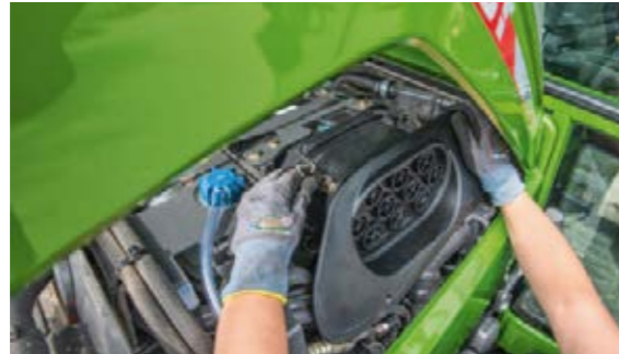
The air filter with Zyklon pre-cleaner stands for maximum performance in air flow and filter life. It is compact, lightweight and particularly well-sealed. Benefit: low maintenance.
