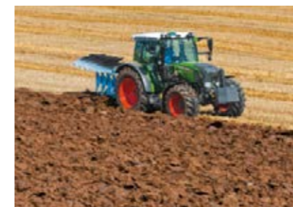
The TMS with built-in Automatic maximum output control 2.0 systematically controls the engine speed and gearbox ratio in the field for best efficiency with differing loads.
