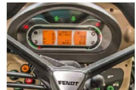
Versatile multi-function display: Display what you need for your work, e.g. the current and average fuel consumption or the worked area.
