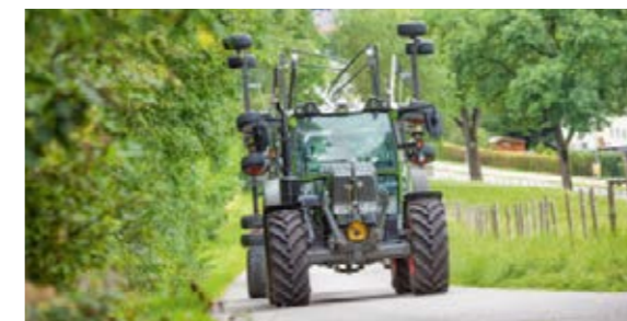
The tractor runs on level ground at a reduced speed. On a slope, the TMS increases engine speed and adjusts the gearbox ratio. As soon as the tractive power requirement is reduced, the TMS reduces the engine speed to the most fuel efficient range possible.
