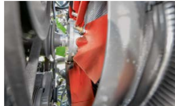
Reverse fans with adjustable fan blades for particularly dusty conditions. Benefit: blow cooling grilles clean without you getting out of the cab – for increased performance and efficiency.
