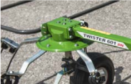
The closed rotor heads are reliably protected against dirt and dust, and feature a long service life.
