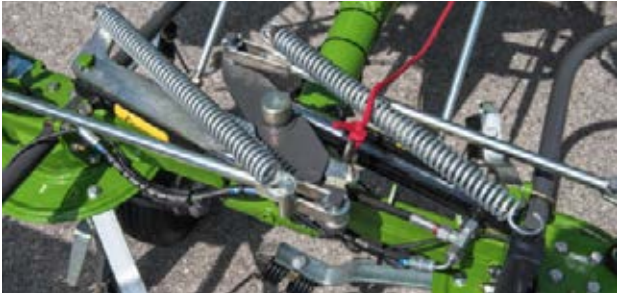
The synchronised lifting ensures safety during folding when working on slopes.
