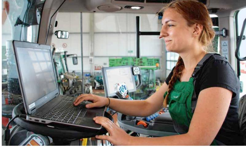
Running diagnostics on the laptop and troubleshooting errors in the electronics. This is now standard procedure in any agricultural equipment workshop, and is therefore an integral part of Lea's training.
