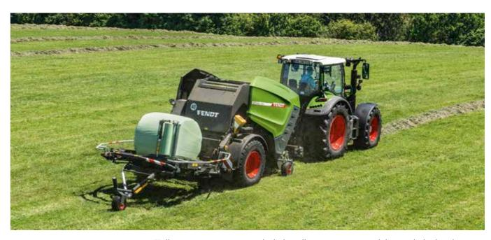
"Following improvements to the baler roller arrangement and the new bale chamber geometry, the Fendt Rotana fixed chamber models are now set to improve forage output, increase bale density, and provide safer bale rotation."
