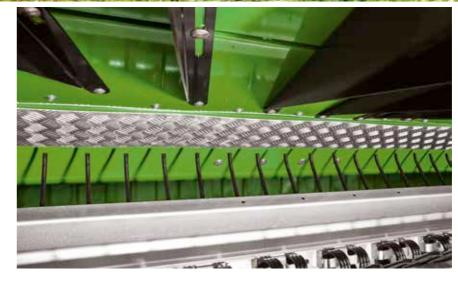
Flexible tines with notching and a checker plate support careful forage pickup and efficient removal of the wax layer on leaves and stalks.
