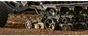
**Tillage discs** Soil types vary widely depending on the region. Various tillage discs are available to suit.
