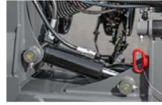
LoadLogic weight management system Hydraulic cylinders can be used to adjust the wing pressure of the Fendt MOMENTUM.
