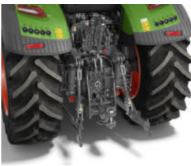
Rear linkage with quick-catch hooks and rub blocks (AU, South Africa, Eastern Europe)
