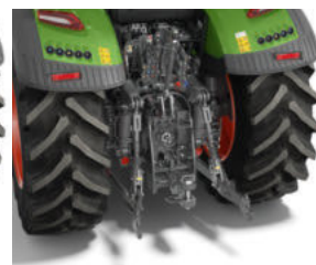
Rear linkage with quick-catch hooks and rub blocks (AU, South Africa, Eastern Europe)
