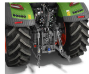
Rear linkage with quick catch hook and side support (EU)
