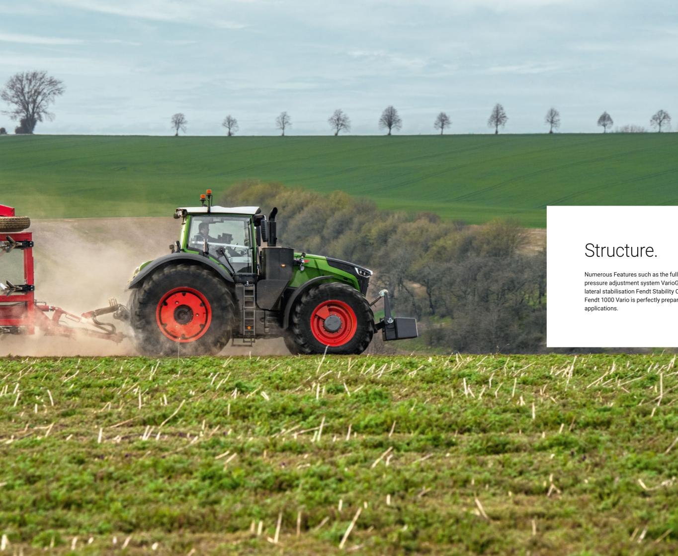
Numerous Features such as the fully integrated tyre pressure adjustment system VarioGrip or the system for lateral stabilisation Fendt Stability Control ensure that the Fendt 1000 Vario is perfectly prepared for a wide variety of
