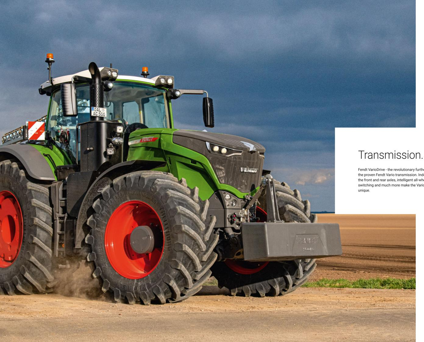
Fendt VarioDrive - the revolutionary further development of the proven Fendt Vario transmission. Independent drive from the front and rear axles, intelligent all-wheel drive, no range switching and much more make the VarioDrive drive train
