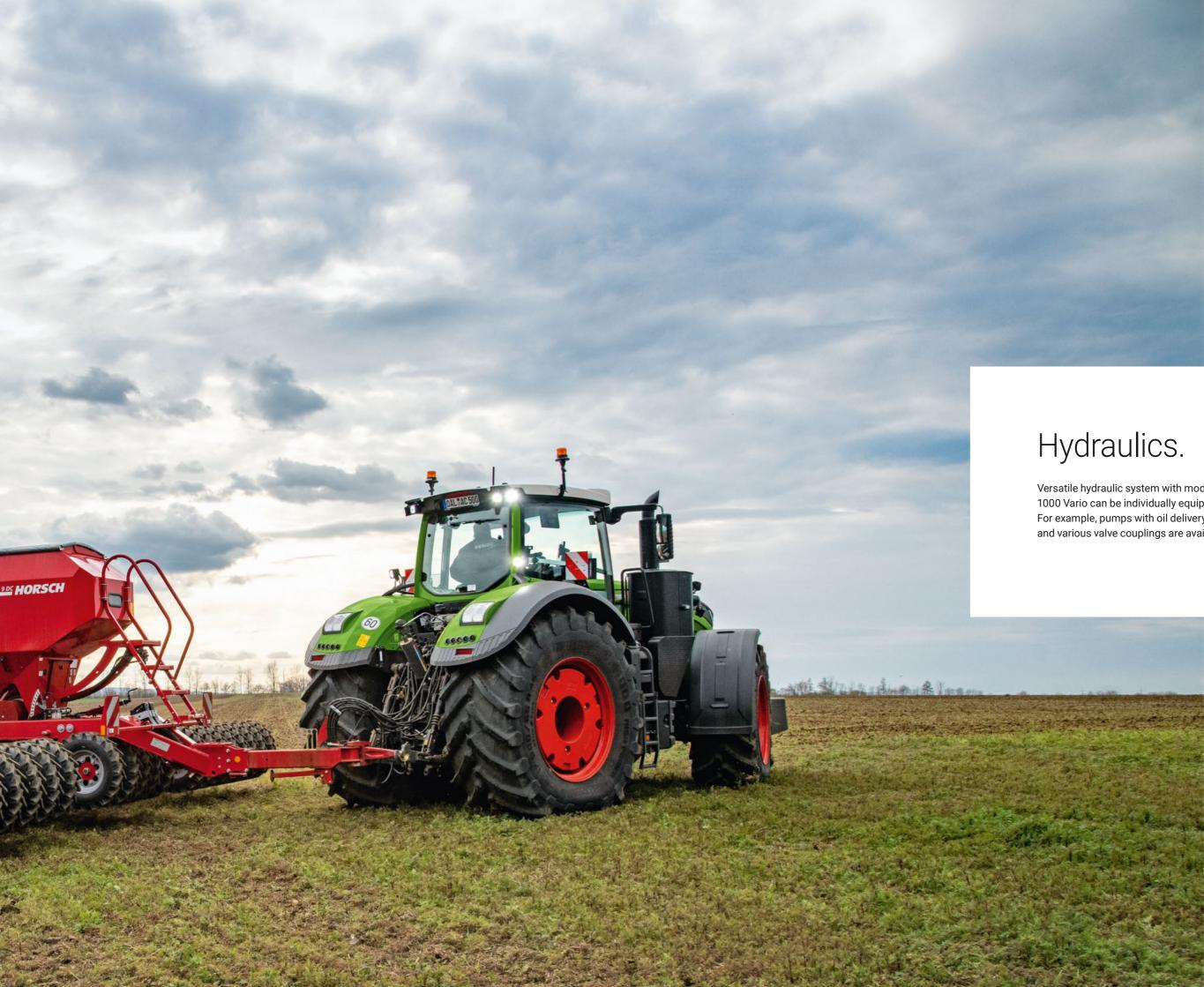
Versatile hydraulic system with modular structure. The  $\ensuremath{\mathsf{Fendt}}$ 1000 Vario can be individually equipped to meet your needs. For example, pumps with oil delivery rates of up to 430 l/min and various valve couplings are available.
