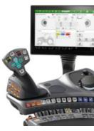
Power+ Setting 1 • No cross-gate lever • Four finger tips (linear modules) for operating the hydraulic valves
