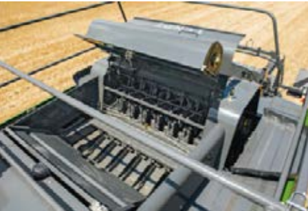
A large maintenance bonnet and foldable traverse-impeller fan guarantee easy access to the knotters.
