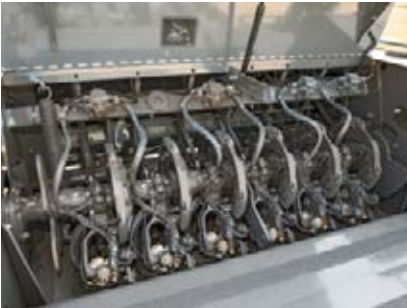
The proven double knotters on the Fendt square balers guarantee reliable tying even under high compression pressure.
