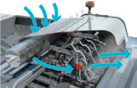
The standard specification cross-flow fan maintains a constant flow of air over the entire knotter area, which thoroughly clears all debris from the knotter area.
