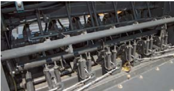
The twine is guided through the knotter brakes for uniform twine feed to the knotter.
