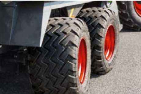
Steering tandem axle for high manoeuvrability.
