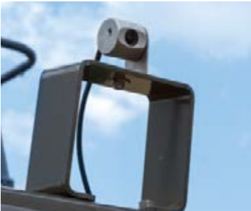
Pre-wiring and a camera port in the terminal come as standard. This means you can install a camera at the end of the baling chamber, for a clear view all around the machine.
