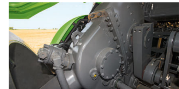
A new high-capacity gearbox is used in the XD baler. Overall, the XD gearbox is 35% heavier than the standard model and can therefore generate even more compression pressure.
