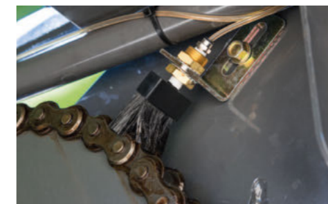
Automatic chain lubrication of all the most important drive chains is new. The lubrication intervals can be conveniently set via the terminal.
