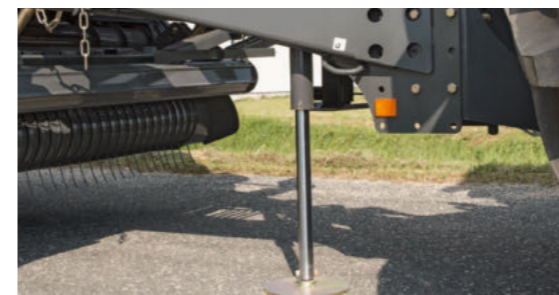
The hydraulic parking jack makes light work of attaching and detaching the tractor.
