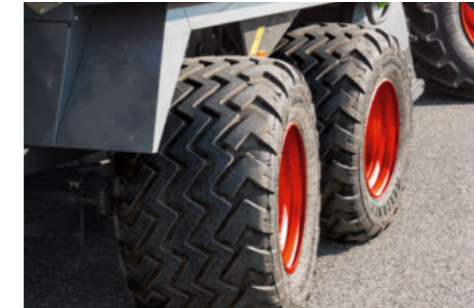
Steering tandem axle for high manoeuvrability.
