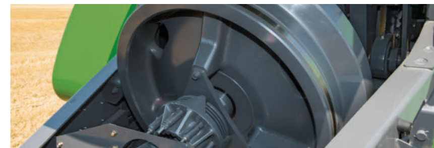
The 545 kg flywheel enables uniform and smooth running, while ensuring high power transfer.
