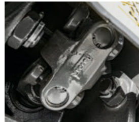
The maintenance-free double-cross joints ensure direct power transfer and means the tedder can turn even in the folded transport position.
