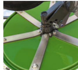
Large rotor plates mean the tine speed remains high at a low rotor speed.
