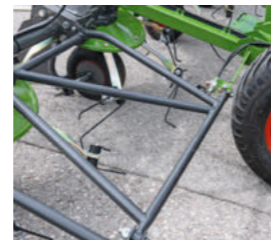
The towed tedders have an extra grid frame for maximum stability, both for protection and to reinforce the main frame across the full machine width.
