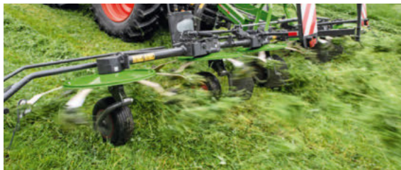
The anti-wrapping system prevents the crop from wrapping itself around the wheel axle.
