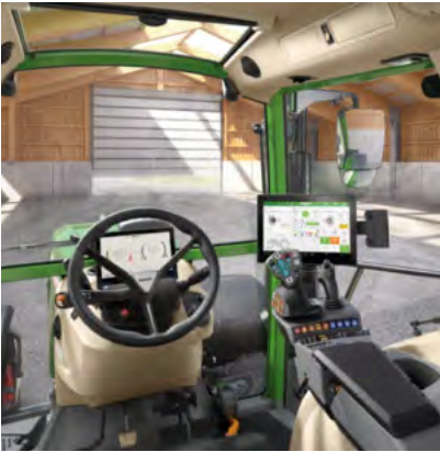
Profi Setting 2 - 3L joystick - 2 linear modules (rocker pair) to control hydraulic valves - 12" terminal
