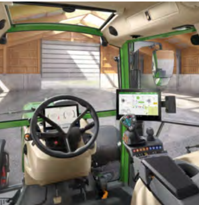
Profi+ Setting 1 - Crossgate lever - 2 linear modules (rocker pair) to control hydraulic valves - 12" terminal
