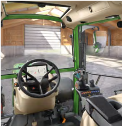
Power Setting 2 - Crossgate lever - No linear module (rocker pair)
