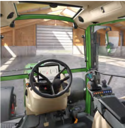
Profi Setting 1 - Crossgate lever - 2 linear modules (rocker pair) to control hydraulic valves
