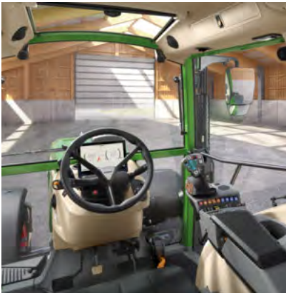
Power Setting 1 - No crossgate lever - 2 linear modules (rocker pair) to control hydraulic valves
