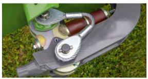
The impact guard protects the mower in the event of a collision, and automatically locks into place again when reversing.
