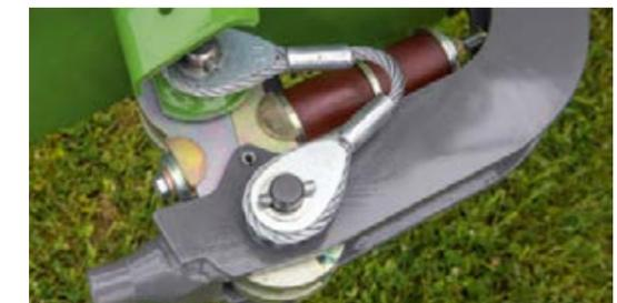
The impact guard protects the mower in the event of a collision, and automatically locks into place again when reversing.
