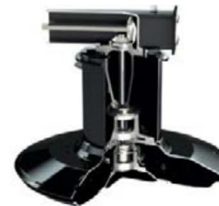
The V-belt drive with automatic tensioning optimises the powertrain function.
