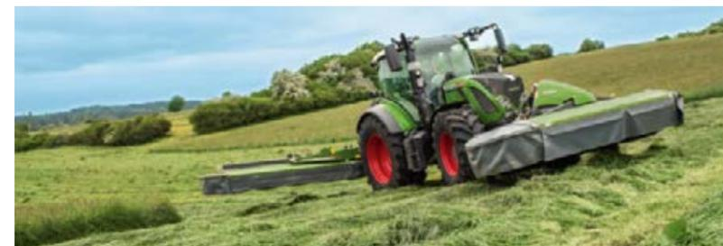
The generous ground clearance enables quick and safe turning on headlands, and the compensating cylinder on the outrigger keeps the mower stable on headlands.
