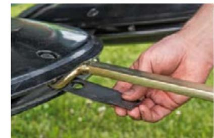
The quick-change system with practical special tool makes changing the knives foolproof.
