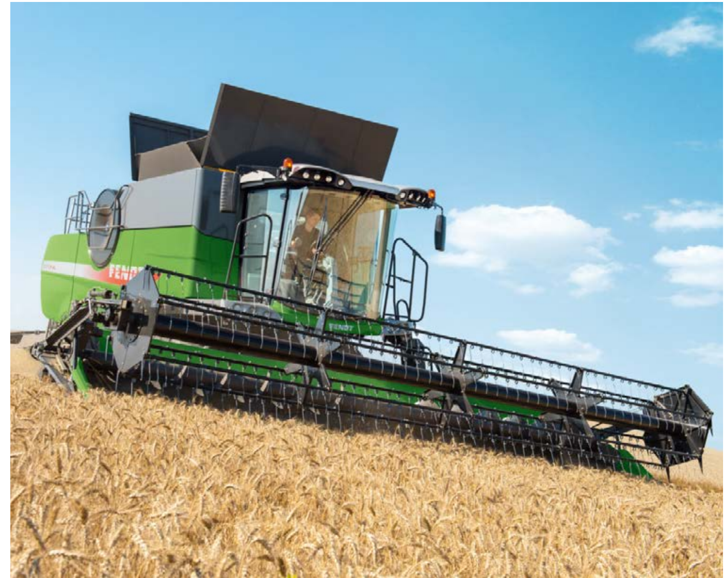
Constant Flow automatically controls the ground speed of Fendt combines dependent on the crop density.
