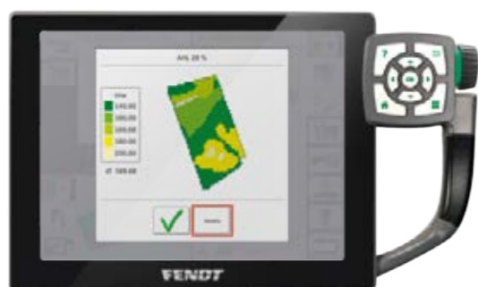
Geo-specific evaluation maps of yields, soil samples, plant nutrient availability etc. can be used to create application maps that reflect actual needs in the field database. These maps then form the basis for section-specific application rates.
