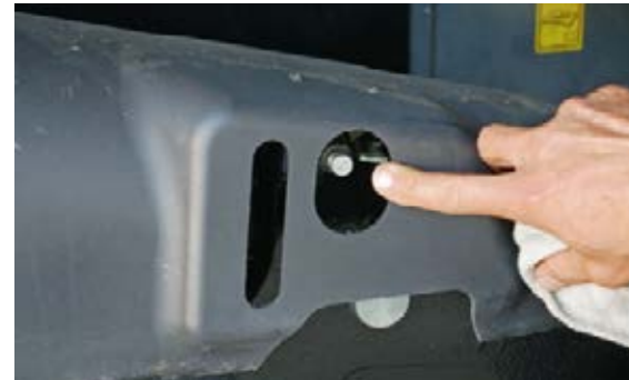
The pressure connections to tension the tracks are easy to access.
