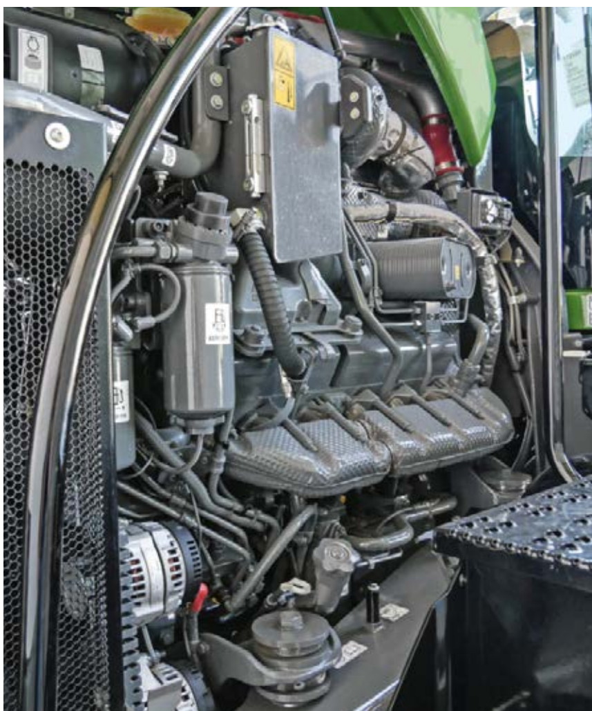
■ The 12-cylinder AGCO Power engine is extremely smooth-running and easy to access for maintenance work.
