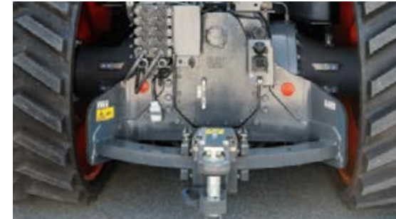
The drawbar, steered hydraulically through 28° on each side, controls the attachments to perfection.
