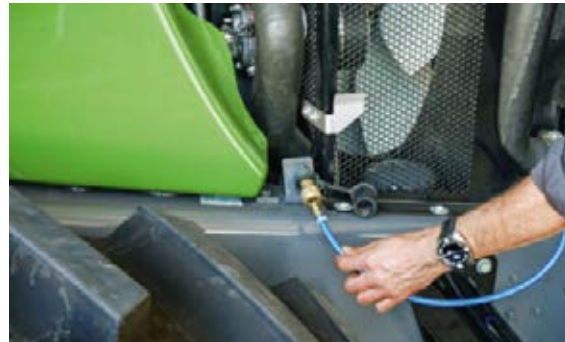
A compressed air connection is located at the front to clean the radiator.
