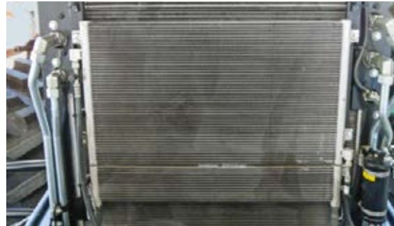
The large cooler units are easy to clean.
