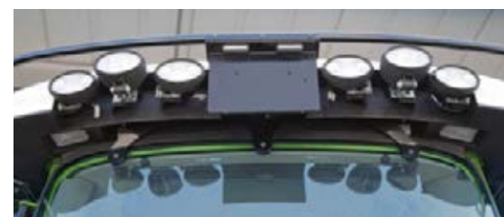
■ Halogen work lights illuminate your surroundings perfectly. An LED headlight is available on request.
