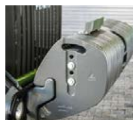
□ Marginal 1996 kg weight can be mounted on the front frame.
