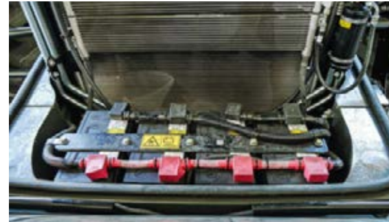
Four maintenance-free batteries supply power in the Fendt 1100 MT.
