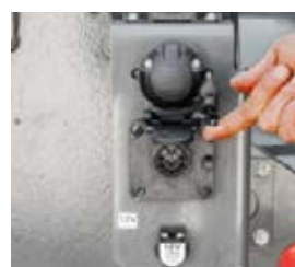
■ There is a 12 V connection at the rear for external consumers. The ISOBUS connection establishes a connection with attachments.
