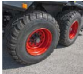
■ The trailing-steered tandem axle guarantees a large contact area with high manoeuvrability.
