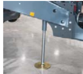
□ The optional hydraulic parking jack makes light work of attaching and detaching the tractor.
