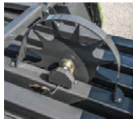
■ Easy adjustment with the electronic bale length control.
