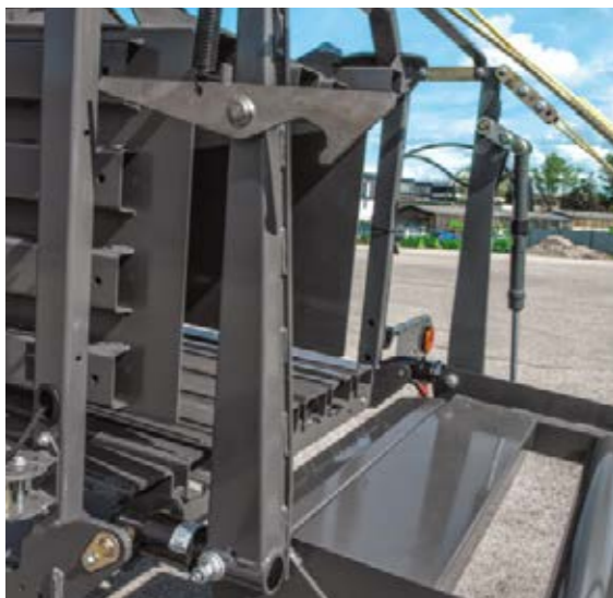
■ The bale load cells between the bale chamber and the bale chute measure the exact weight of the bale and send the data straight to your terminal. The system is protected by the integrated wiring set in the chassis and hence the cables are not easily torn.
