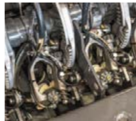
■ All knotters and important drive chains are lubricated automatically, and the lubrication interval can be easily set on the terminal.
