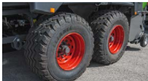
■ The Fendt Squadra 1290 UD comes with 2 different tyre options for an external width of less than 3 metres: 620/50R22.5 and 620/55R26.5.
