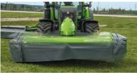
The +/- 5° swing means that the Fendt Cutter FPV can be adjusted to the ground, and that no stalk is left behind.
