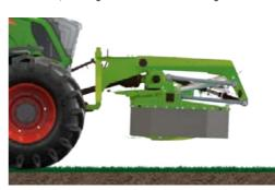
The Fendt Cutter FZ drum mowers with headstock adapt perfectly to the terrain with a maximum stroke of 490 mm, and are gentle on the soil with their large bearing surface.
