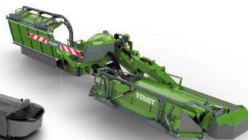
Mower combinations with ISOBUS Complete automation with grouper belts Working width 9.30 m
