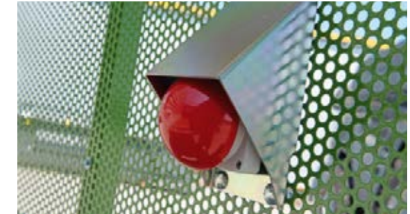
And an optional acoustic level indicator is controlled by a capacity sensor on the rear wall.
