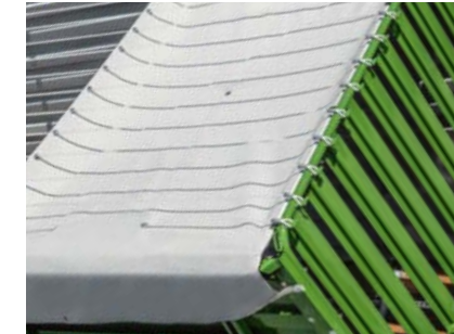
The optional tarpaulin curtain at the front keeps the feed securely in the loading space.
