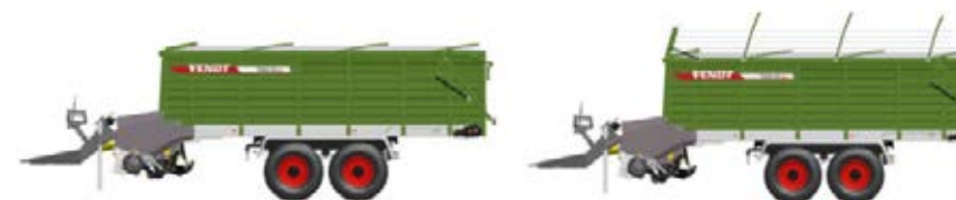
The collapsible dry feed assembly can be folded in and out from the cab. Transiting is therefore no problem, and for hay harvesting the loading space can be quickly extended.
