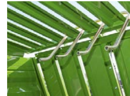
With the two-stage automatic loading system, light pressure is applied via a gauge bar, while moderate pressure is applied via the loading flap.
