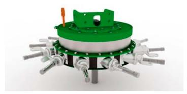
The rotor is integrated in the existing housing of the rake socket as an external rotor.
