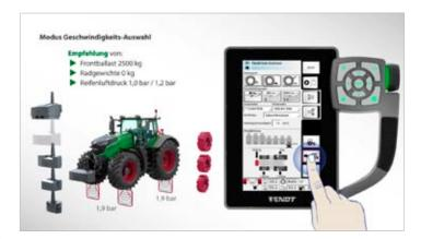
Adapted ballasting and correct tyre pressure are decisive variables in minimising power loss due to slip and rolling resistance.
