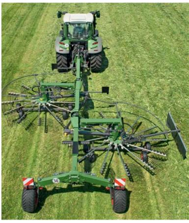
other. On the Fendt Former 12555 X, however, it is possible to adjust the speed on each rotor separately – independent of the engine and ground speed of the tractor. This makes it possible to react quickly and individually to the different structures of the forage crop.
