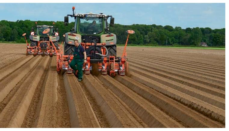
The machine combinations each pull four dams with carrot seeds precisely with VarioGuide RTK.
