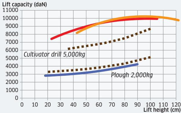
Fendt 724 Vario: As the lifting force steadily increases, the tractor has no problems hoisting the heavy cultivator drill. Also, the 724's lift travel is more than 80cm.
