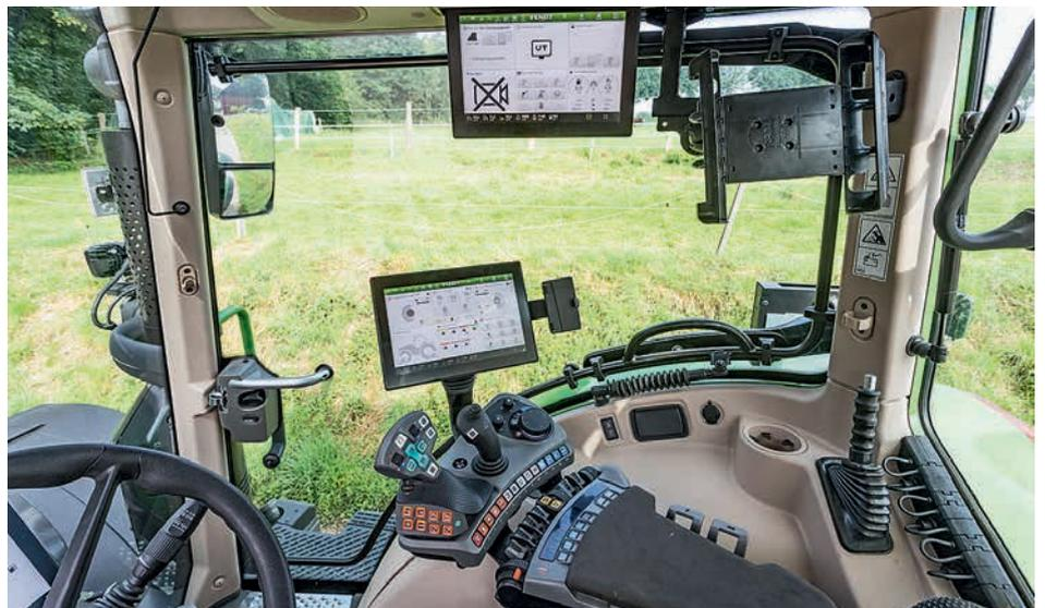
The armrest is completely new on the 724. Also new is the additional display up in the roof, which can be pushed part-way into the roof to improve the to-the-side visibility when on the road.
