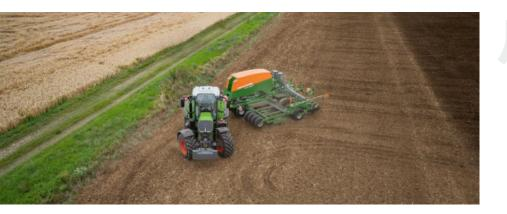
Yet we were even more impressed by the 728's manoeuvrability. Thanks also to the, pull-inturn' effect of the automatic all-wheel drive, we measured a turning circle of just 12.25 m (VF600/70 R30, 1.98 m track width) - that's very good!" (profi 3/2024)
