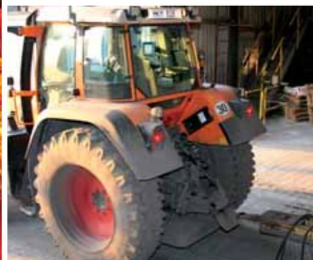
Modifications: With the heavy-load hitch and additional ballast under the tractor, the 714 Vario is well-prepared for towing heavy loads.
