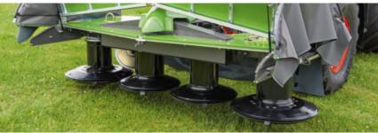
Smooth-running guards which swing upwards make a huge difference to cleaning and maintenance. All Fendt Cutters are very easily accessible.
