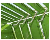
With the two-stage automatic loading system, light pressure is applied via a gauge bar, while moderate pressure is applied via the loading flap.
