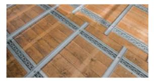
With the four 10 mm thick round steel chains of the large Tigo MS, MR and all MR Profi models, with 50 t breaking load you are prepared for even the toughest applications. The small Tigo MS and MR models provide support with two scraper floor chains and 25 t breaking load. You can also opt to equip the smaller models with four chains and offset scraper bars.
