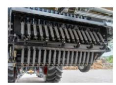
Get set up quickly and easily under all conditions, whether for feed, hay or silage, by adjusting the number of knives to 0, 5, 17, 21 or 33.
