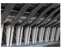
The single-section conveyor swing arm allows an even and smooth forage flow.
