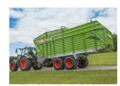
All Tigo MS and MR models have a permissible maximum weight of 12 t. You can opt to increase this to 15 t on Tigo MS models and to 17 t on MR and MR Profi models.
