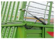
Another option is to have the collapsible dry feed assembly folded in and out hydraulically.
