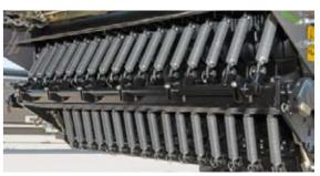
You can also opt to have the cutter unit pivot hydraulically from its working position to service mode.
