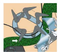
The double tines remain in contact with the crop at an ideal angle until they are retracted in a horizontal position just before the crop enters the loading space.
