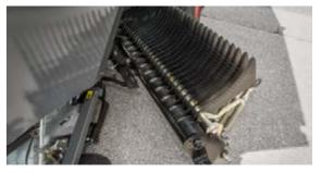
The central knife release allows you to change individual knives quickly and easily.
