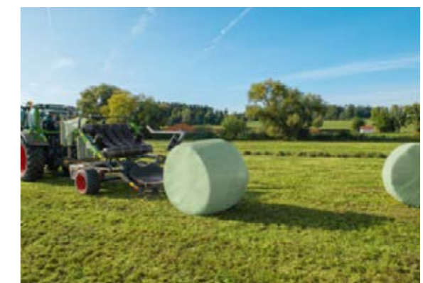
The Rollector 160 is equipped with a bale unloading table with active drop – this effectively avoids damage to the film.
