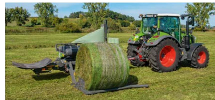
Both the loading arm and the wrapping table can be adapted to different bale sizes. Safely pick up bales with a diameter of 1.25 m to 1.6 m and pack them airtight in film.
