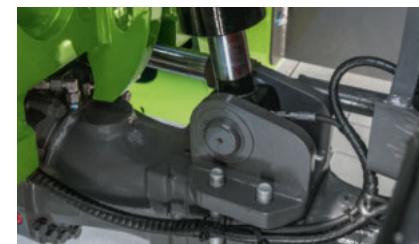
Chassis Options Pendulum axle lock for the rear axle • Function 1: swings free • Function 2: automatic activation at standstill • Function 3: permanently locked
