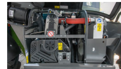
Cooling - Options • Reversible fan • Activation automatically in 3 intervals (20, 40 or 60 min.) or manual activation via a button
