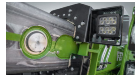
Dirt scraper • Prevents dirt from entering the interior of the telescopic boom and damage occurring
