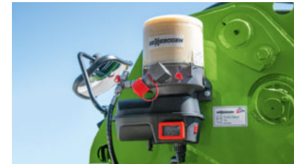
Central lubrication • Supply of all lubrication points including those on the telescopic head
