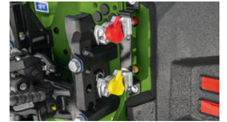
Assembly - Options • Compressed air brake system
