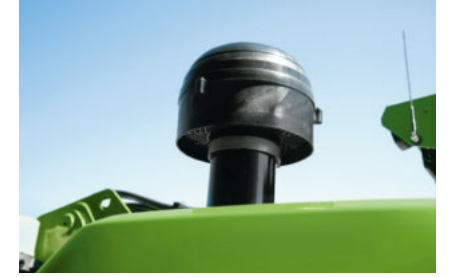
• Cyclone pre-separator for the air filter (up to 98% separation)
