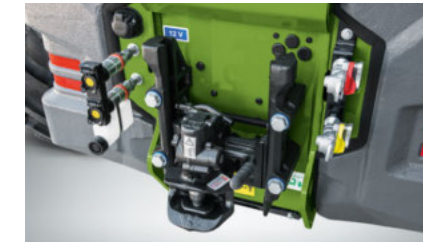
• Automatic trailer coupling (Rockinger) • Maximum trailer load: 18.5 t
