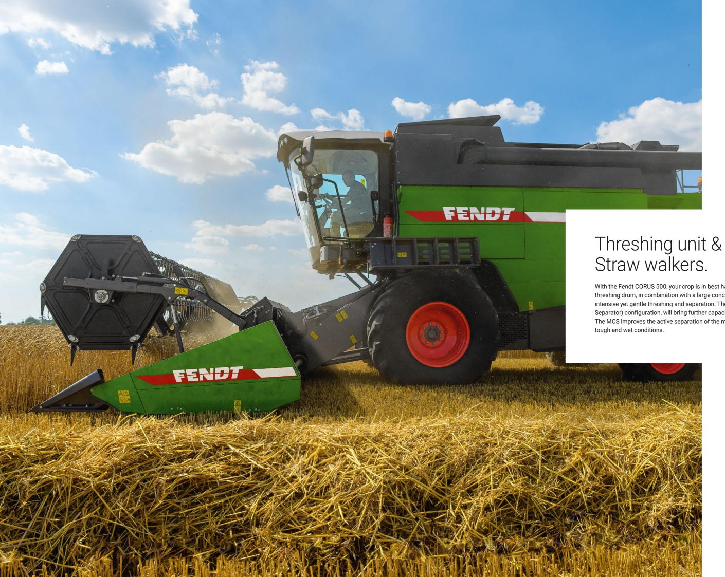
With the Fendt CORUS 500, your crop is in best hands. The powerful threshing drum, in combination with a large concave area, ensures intensive yet gentle threshing and separation. The MCS (Multi Crop Separator) configuration, will bring further capacity to your operations. The MCS improves the active separation of the machine especially in
