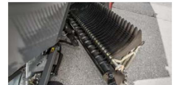
The central knife release allows you to change individual knives quickly and easily.
