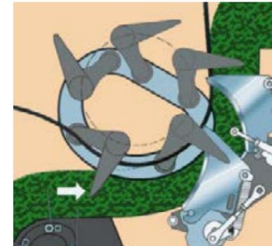
The double tines remain in contact with the crop at an ideal angle until they are retracted in a horizontal position just before the crop enters the loading space.
