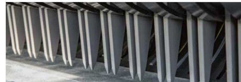
The short distance between the pick-up and the loading unit allows an optimum crop flow.
