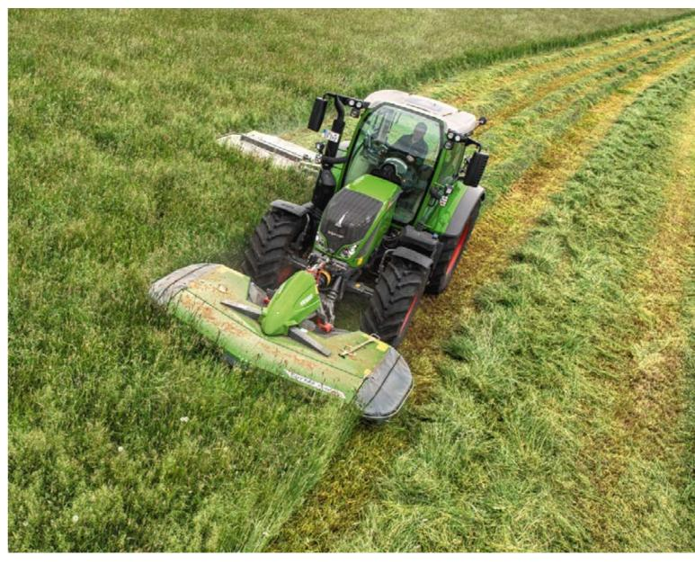
The +/- 5° swing means that the Fendt Cutter FPV can be adjusted to the ground, and that no stalk is left behind.
