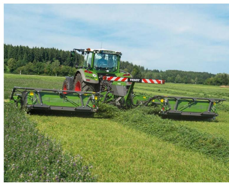
The belts can be folded down and the crop discharged in the swath across the required width at the touch of a button The belt speed can be adjusted at the touch of a button on the Varioterminal.
