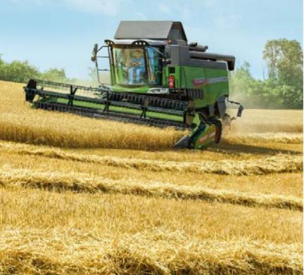
Our C and L-Series combine harvester models are available in a ParaLevel version. The system is based on a parallelogram and compensates for slopes up to 20%.
