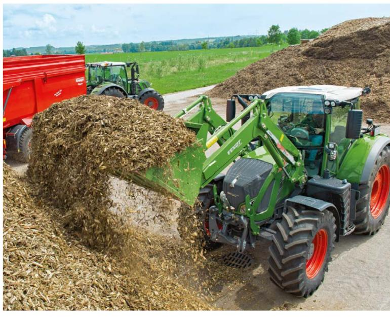
High-performance load-sensing hydraulic systems in Fendt Vario tractors makes it much easier to operate the front loader.
