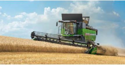
All models of the Fendt X-Series and P-Series are available in an AutoLevel version. The integral rump levelling system, which pivots the final drives, levels the entire machine is levelled on slopes.
