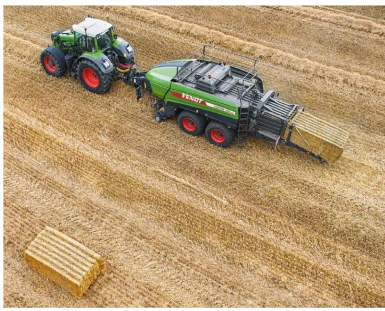
In order to handle the changing requirements of customers and to make long transport routes profitable, the Fendt Squadra 1290 UD has been designed so that it can produce bales with 20% more weight as compared to existing big balers.
