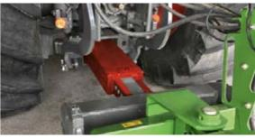
These tractors offer up to 10 kW of electrical power for attachments. The interface that is used is the easily modifiable AEF high voltage interface.
