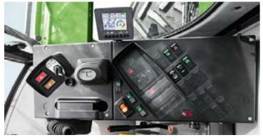
You can control the entire combine using the side console of the Fendt E-Series. The digital on-board computer displays the running machine data. In addition to gear shifting, you can also operate the lights and speeds for the engine, threshing cylinder and blower here.
