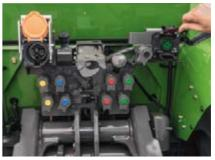
Front-mounted devices can also be driven hydraulically, electrically or by PTO.
