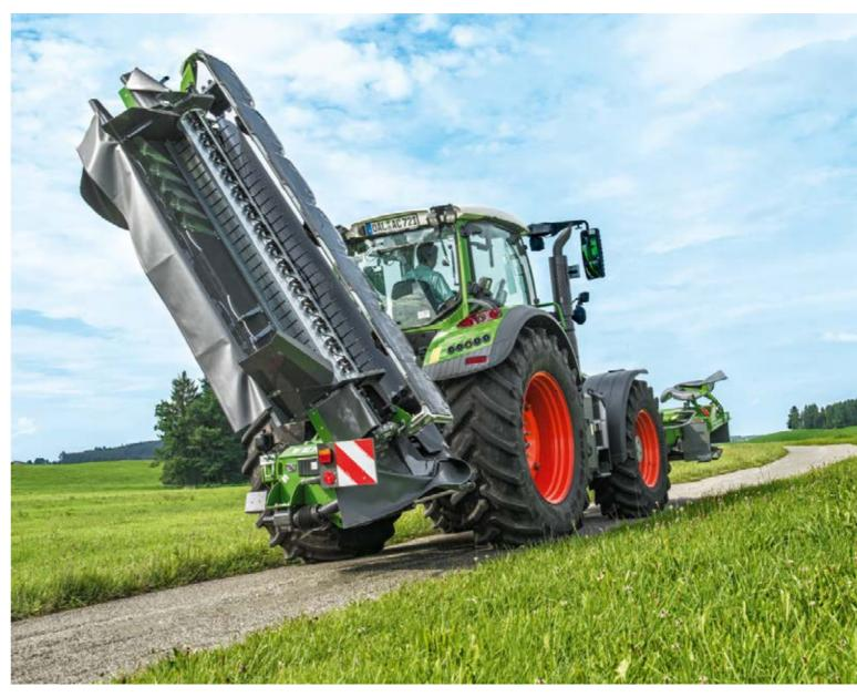
Through perfect weight distribution and the wide folding angle, tractor and mower merge into one unit on the roads.
