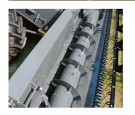
The FreeFlow table has feed fingers over the entire width, which increase the output of the intake auger and guarantee active, fast feed into the crop elevator.
