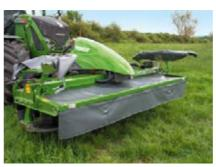
The unique patented SafetySwing impact guard can swing the mower combination up and to the rear, if necessary by up to 1.5 m.
