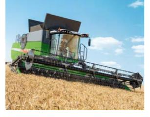
The Schumacher cutterbar is tried and trusted a thousand times over. With 1,220 cuts per minute, it always ensures a clean cut. The knives are arranged alternately, so the cutterbar is self-cleaning and always remains sharp.
