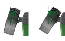
In relation to the default setting, with VarioActive you only need approx. 60% fewer turns of the steering wheel to achieve the samewheel lock. With VarioActive, you profit through the faster reaction of the steering during tight turning manoeuvres at the headlands.
