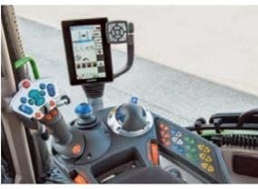
You can control ISOBUS-capable implements via the Variotronic Implement Control, directly with the joystick or Varioterminal. So you do not need additional terminals in the cab.
