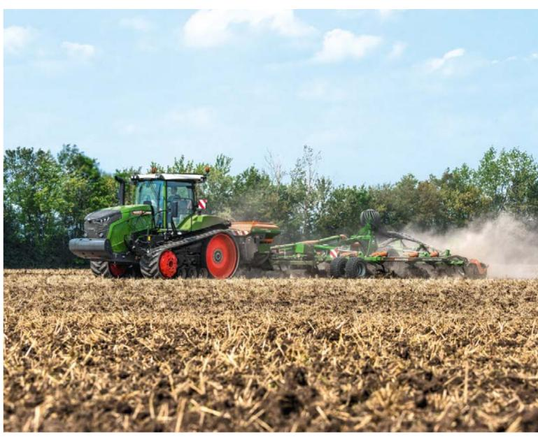
The middle rollers are spring-mounted by ConstantGrip in order that ground contact is not lost and power can be Even on headlands, the Mobil Trac System shows its strength and does not create deep tracks. Variotronic<sup>TI</sup> headland management saves you the time and trouble
