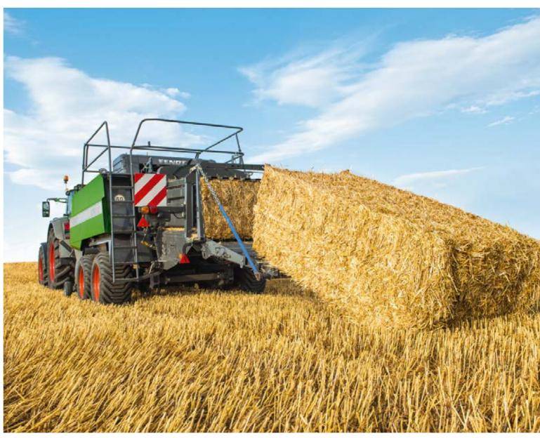
A new roller pressure pad and a large deflector plate ensure uniform crop flow into the baler.
