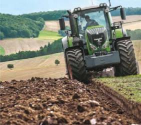
The front axle suspension of the Fendt 800 and 900 Vario offers enormous comfort at 60 km/h not only on the roads. The front axle, which has been specially adjusted for field work, never loses contact with the ground and therefore provides exceptional traction.
