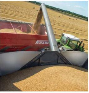
The grain tank capacities are adapted to the high machine output and have a capacity of up to 12,500 litres. That guarantees high efficiency, longer threshing times and therefore more time for harvesting.
