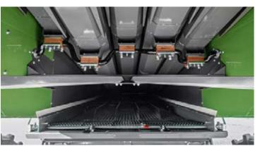
The so-called active, open rear walls of the steps further improve residual separation.
