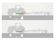
Shifting the static and dynamic loads from the rear axle to the front axle enables a high and evenly distributed traction transfer.
