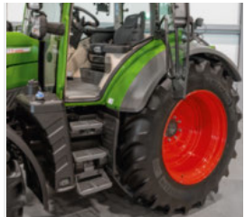
■ The entrance is protected against dirt from the side. There are also wide steps and a well-placed handrail to get up and down safely. The door handle is easy to reach from the ground.
