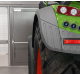
Full wheel protection with extra-wide mudguard at the rear and side – keeps out the dirt
