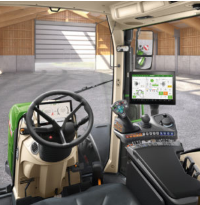
Profi+ Setting 1 - Crossgate lever - 1 linear module (rocker pair) to control hydraulic valves - 12" terminal
