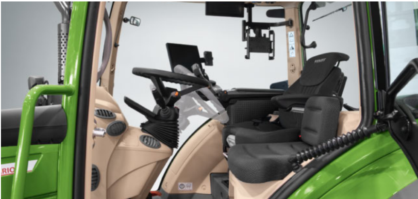
Perfect ergonomic adjustment: The steering wheel and cockpit are easy and quick to adjust with the foot pedal. For the best sitting position, the steering wheel and cockpit must be at the right height and tilt angle. Benefit: The best view and minimal glare in the cockpit. For a comfortable exit, just pivot the steering column and cockpit upwards with the foot pedal.
