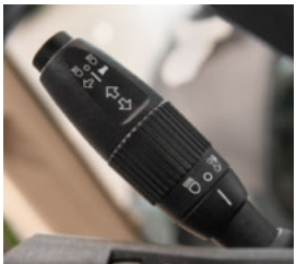
■ Particularly practical and as comfortable as a car: the indicator reset has 3 trigger settings: steering angle, time and speed.
