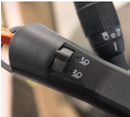
■ Two programmable lighting modes: use the switch on the reverse lever to quickly toggle between two stored lighting modes, including road and field mode.
