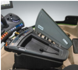
■ Fold-away compartment under the armrest: as well as providing storage, this houses up to 4 USB sockets so you can charge and run your devices.
