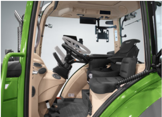
Perfect ergonomic adjustment: The steering wheel and cockpit are easy and quick to adjust with the foot pedal. For the best sitting position, the steering wheel and cockpit must be at the right height and tilt angle. Benefit: The best view and minimal glare in the cockpit. For a comfortable exit, just pivot the steering column and cockpit upwards with the foot pedal.
