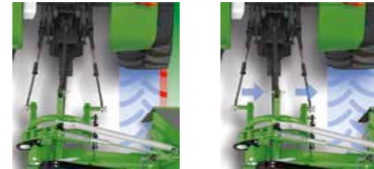
■ Full utilisation of the working width through adjustable lower link pins.
