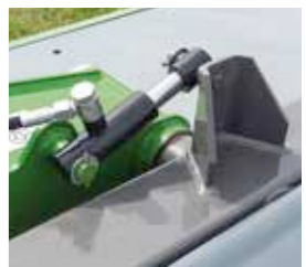
■ A compensating cylinder prevents the mower unit from swinging at the headlands or when driving on the road.
