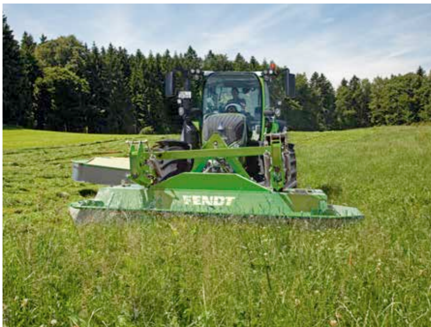
■ Torsion-resistant cutter bar with welded U-profile. □ Additional swath discs can reduce the width of the swath to a narrow 0.65 m.
