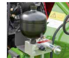
■ Floating cut: The TurboLift System permits adjustment of the contact pressure on the cutter bar (hydropneumatic relief) while driving.
