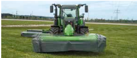
■ Perfect adaptation to the ground thanks to 5° pivoting angle side-to-side as well as springs or load relief front linkage control in the direction of travel.
