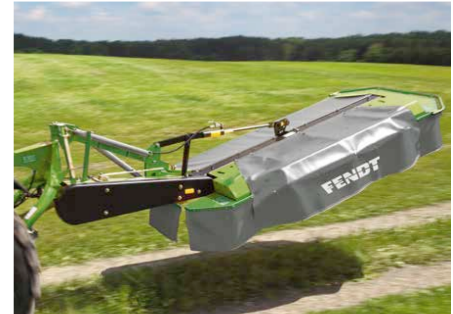
■ The mower can be swung in behind the tractor from the comfort of the driver seat.
