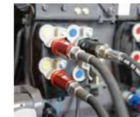
■ Typical Fendt: readily visible and permanently colour-coded hydraulic hoses.
