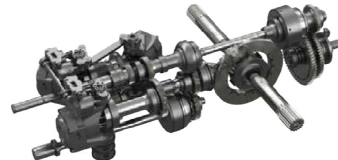
The Fendt Vario transmission is a hydrostatic-mechanical power split drive. With increasing speed, the share of the mechanical power transmitted through the planetary set increases. The hydrostats can be swung 45 degrees and have a high operating pressure of max. 550 bar – this ensures exceptional efficiency.
