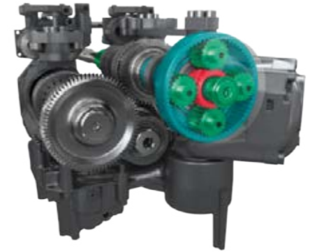
The transmission on the top models over 330 hp have been designed for the highest loads. It has a set of four planetary gears, which optimises power transfer and results in high robustness.
