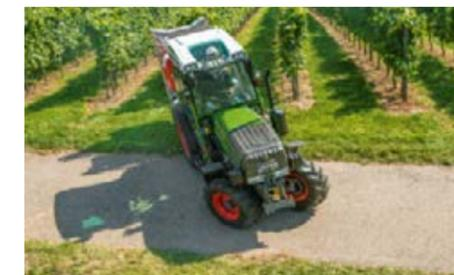
The streamlined wasp-waist design allows a wide steering angle up to 58° and outstanding manoeuvrability in combination with the VarioActive steering system.
