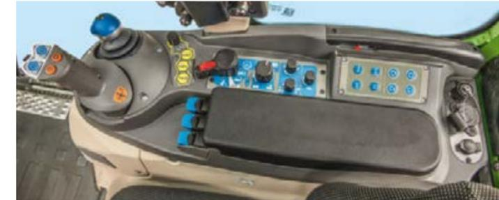
The steering console is adjustable in width and is adapted to your seat position.
