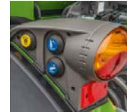
■ The required PTO speed can be conveniently selected via the rotary control.
