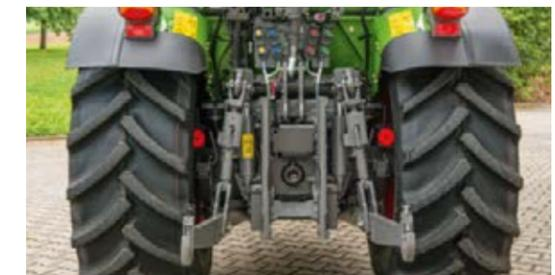
A fully-fledged Cat2 power lift is available in the P-variant. All connections are clearly arranged and easily accessible on all variants.
