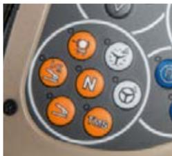
The VarioActive superimposed steering system and the Guidance system can be conveniently activated on the steering wheel console.
