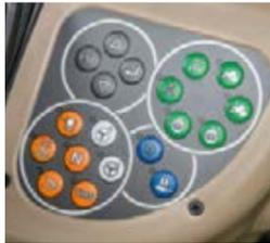
On the dashboard, you can quickly and easily operate the multiple display, comfort engagement for 4WD, differential lock and front axle suspension as well as the Tractor Management System TMS.
