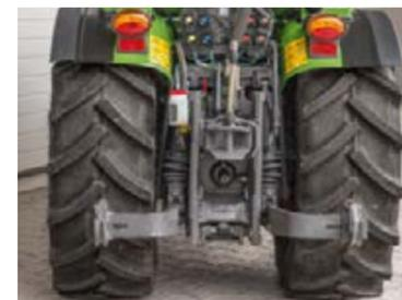
The swinging power lift on the V/F variants is linked in front of the rear axle. The width-adjustable lower links and hooks allow simple adjustment to match any implement.
