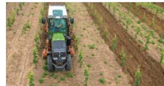
The smallest turning radius is just 3.2 m, depending on the tyres. You will notice this immediately at the end of the row, where you can switch to the row after the next without having to change direction.
