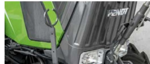
□ The hydraulic hoses are always neat and clutter-free thanks to fasteners at both sides.
