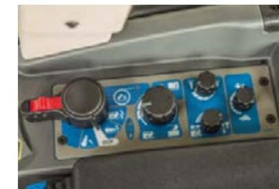
The rear power lift can be easily adjusted in the EHR control panel. The button can be transferred to the multi-function joystick with the automatic function.
