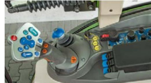
In the standard version, the Fendt 200 V/F/P Vario is controlled via Vario Joystick which also has an engine speed memory button and the cruise control memory button.
