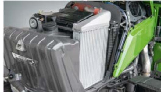
The U-shaped cooling system has large intake areas with optimum air supply. This results in a low cooler contamination even in extreme usage conditions.
