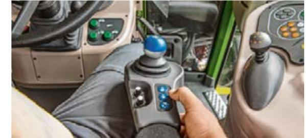
At the headland or during front loading work, you benefit from VarioActive steering, reaching a full wheel turn with just one steering wheel rotation. Up to 8 km/h the superimposed steering system is unrestricted, from 8 to 18km/h the superimposition effect is linear.
