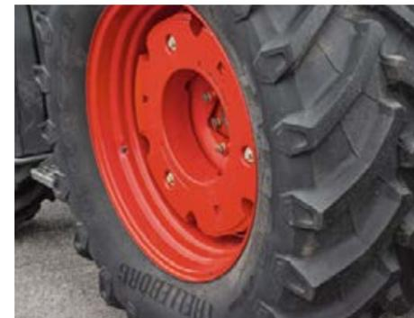
Universal weights round off the ballasting system and stability against overturning perfectly.
