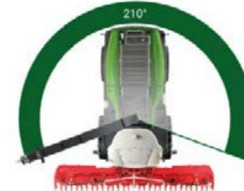
Even with an unloading height of over six metres, operators have the chute flap in full view. Optionally, the discharge chute can be extended to permit the loading vehicle to be filled optimally, even with wide headers.
