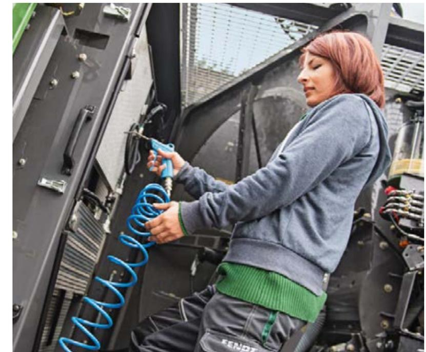
The components on the Katana are especially easy to access thanks to large maintenance flaps, which open upwards, not sideways. The maintenance lighting makes all the difference in the dark.
