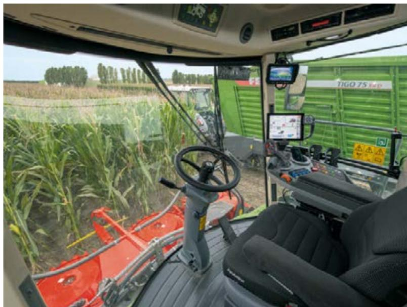
The Visio5 cab has been designed for optimum visibility and offers perfect ergonomics and easy-to-use controls in the workplace. Thanks to the special shape of the roof line, operators always have the chute flap in view. Automatic climate control and heating guarantee a pleasant working environment.
