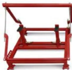
Assembly support for easy, fast assembling and disassembling of the chopping assembly for cleaning and maintenance.
