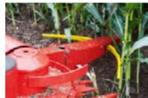
Thanks to the row sensors on the tips of the maize header, the Katana works through the crop very precisely and fully automatically.
