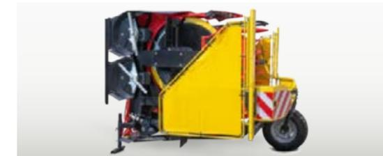
With the 460Plus attachment in the StalkBuster version, the corn stubble can be crushed even during harvesting. Perfectly equipped against an infestation of corn borers.
