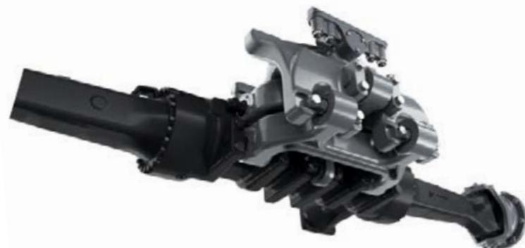
The rear axle has suspension to absorb shock loads in the field and on the road. That protects both the operator and the machine. The suspension also enables better ground contact for the Fendt Katana and boosts pulling power. Together with permanent 4WD as standard, this means the best propulsion.
