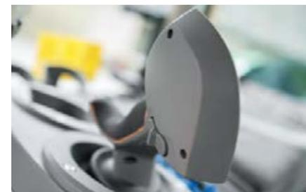
The roller pressure pad on the pick-up is easy to operate with the rocker switch on the back of the multifunction lever. It allows you to pivot the swinging frame manually for maize work and actuate the indicator in road mode.
