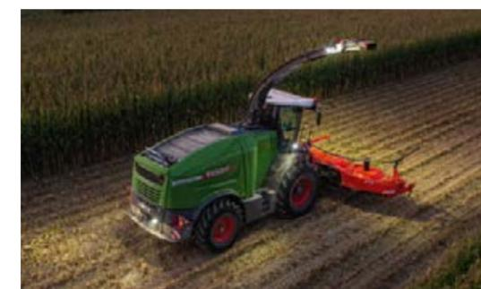
Well thought-out positioning of the LED lights facilitate work around the machine at dusk or when dark and save energy.
