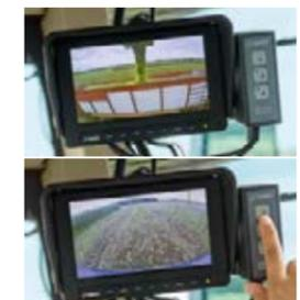
When driving forward, you can see the fill level of the accompanying vehicle through the camera on the discharge chute. When reversing, the image is automatically switched to the reversing camera.
