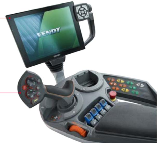
The 10.4" Varioterminal with colour display and touch screen (rotary control and keys also possible) is easy to use and guarantees full machine monitoring, to keep the machine working reliably.
