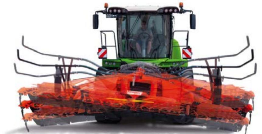
Together with the innovative swinging frame directly on the intake, ground-contact sensors actively adapt the header to the ground contour.
