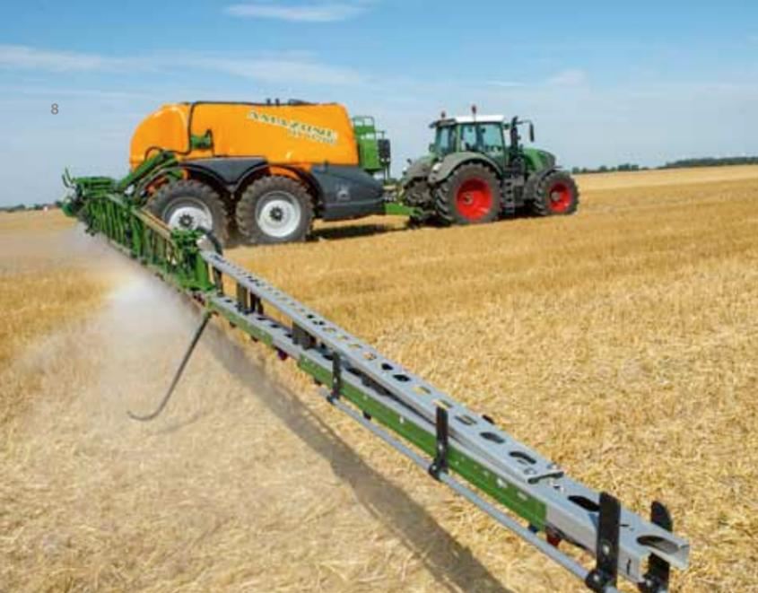
Fendt 800 Vario with SectionControl: section control via fully automatic GPS signal.
