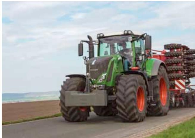
Fendt 800 Vario: The self-levelling front axle suspension ensures excellent ride comfort.
