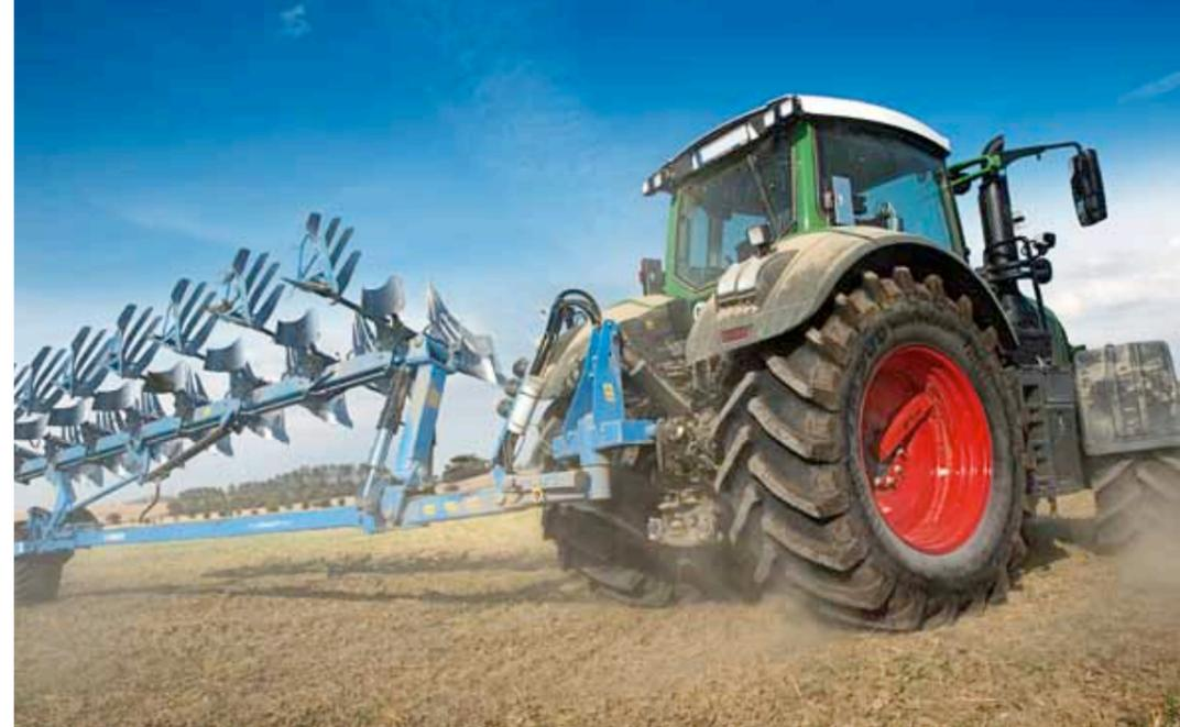
Lowering the tyre pressure with VarioGrip provides more pulling power.
